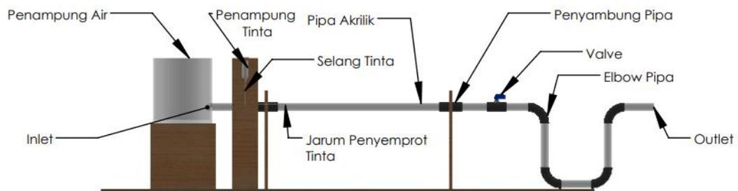
**Gambar 4. Skema instalasi *water tunnel***
